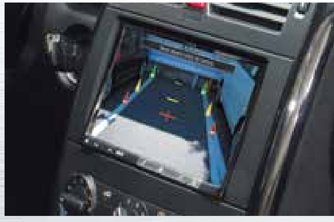
A rear view camera is a great way to improve your parking skills and make reversing safer. The camera image automatically comes on when you shift into reverse, and distance guides that can be adjusted to match your car size help when parking. The cameras are very small, so they're easy to install and don't change the appearance of the car.
